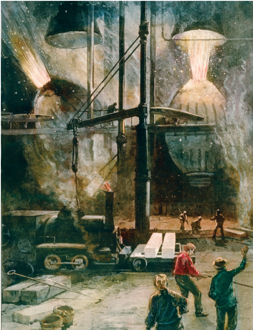
This engraving of steel manufacturing at Andrew Carnegie's plant in 1886 features a Bessemer Converter, which converts molten pig iron into steel. The process was named after Sir Henry Bessemer of Sheffield, England, who first patented the process in 1855.
